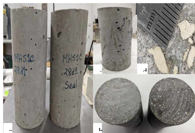
Figure 3 Image of a) Unsealed and Sealed hemp-concrete samples b) top view of sealed and unsealed samples c) cracked sample on 28 days d) magnified image of hemp shives in concrete
