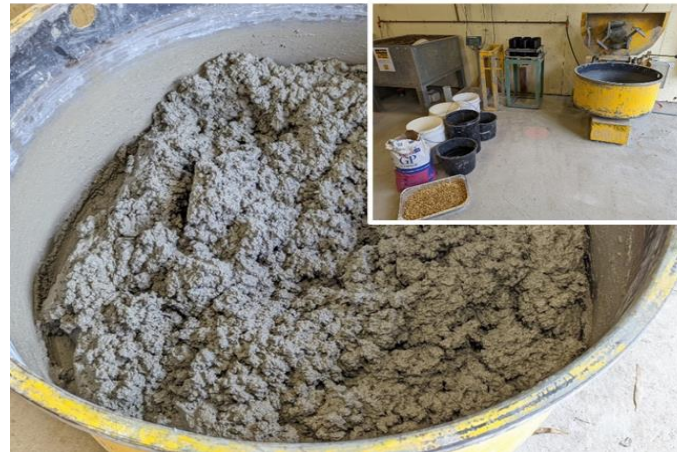
Figure 1 Batch mixing hemp-concrete composite
