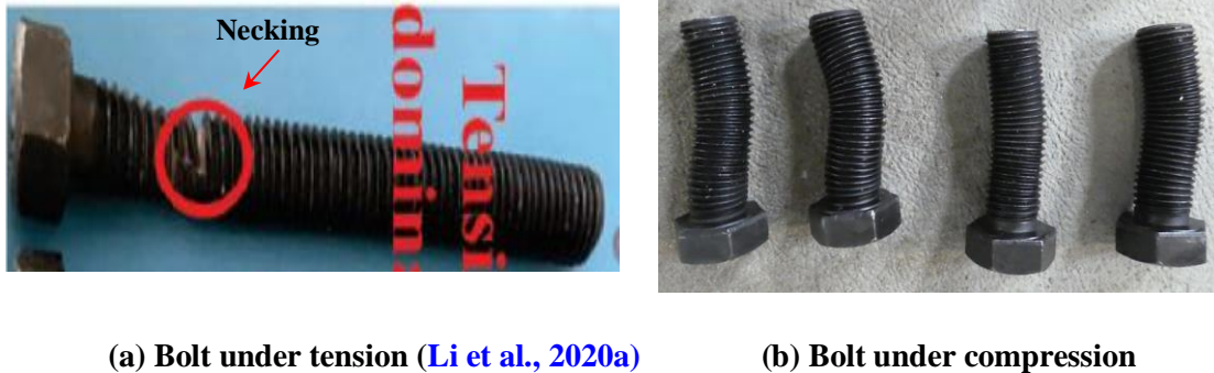
Figure 3. Failure modes of bolts under tension and compression
