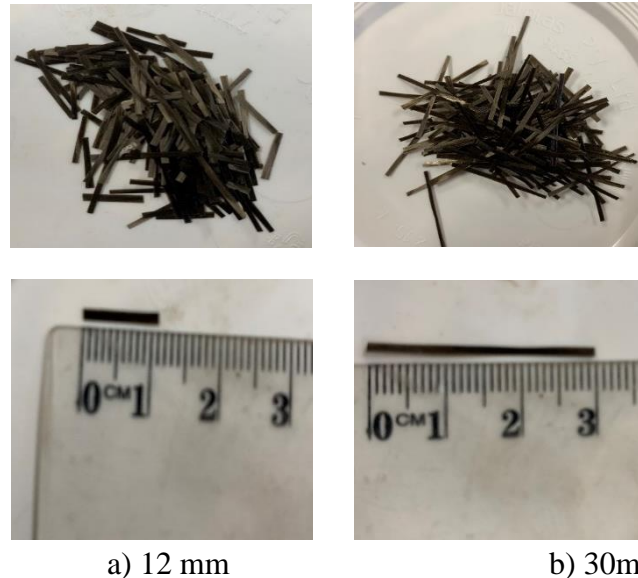
Figure 1. Short basalt fibres with 12 mm and 30 mm were used in SCGC [42]
