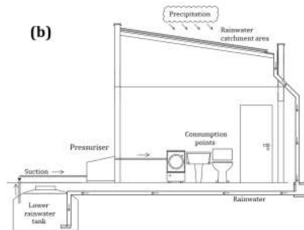
Figure 1. Indirect (a) and direct (b) rainwater distribution schemes
