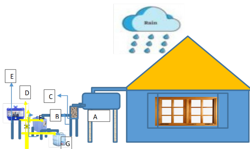
Figure 1. Schematic diagram of the field setup, A-Rainwater tank, B-Filter, C-Solenoid valves, D-Corrosive graded solenoid valve, E-Pool chlorine tank (15Liter), F-Disinfection Tank, G-Storage tank.
